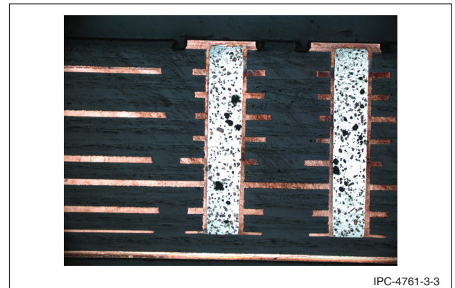
Figure 3-3 Voids in Via Fill Material
